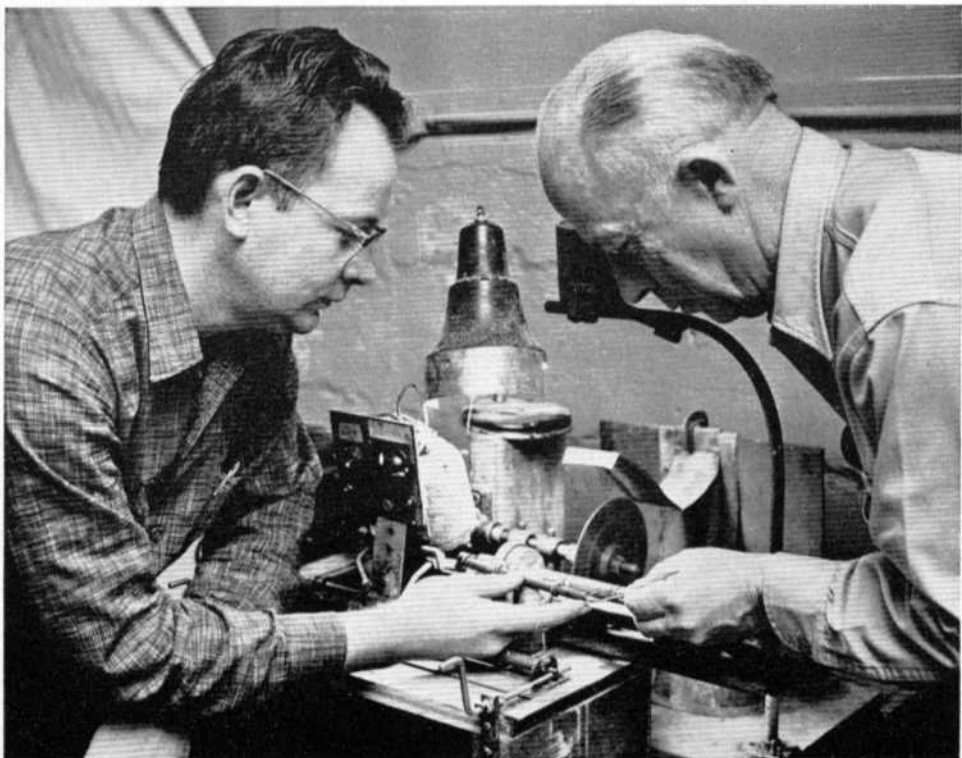
Above: Elroy Peterson and Oscar Merwin using lathe for cutting jade shafts. Lathe devised by Peterson and Paul Baer.
