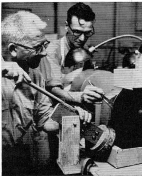
On left above: Alden Clark using a special device for sawing the curved face on pendulum bob. Robert Hardenbrook puts coolant on the saw.
